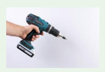
Figure 11.3: The 'trigger' on the hand drill is a small-scale dead man's switch
