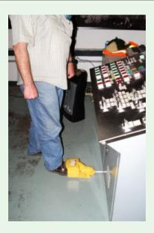
Figure 11.4: A worker must have their foot pressing the 'dead man's switch' for the control panel to operate
