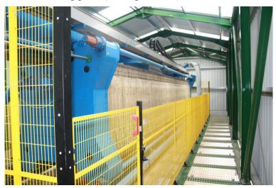
Figure 11.2: Moving parts of a machine are guarded by a yellow safety fence
