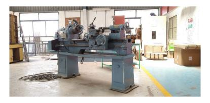
Figure 11.5: An industrial lathe machine
